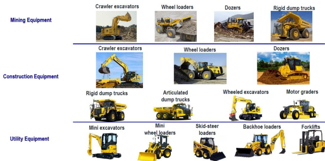
Figure 10 Examples of Off-Road Vehicles – Mining, Construction and Utility equipment
