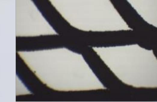
Electrosprayed grid with HSAG graphite in a current collector grids used in air-breathing PEM fuel cells.
