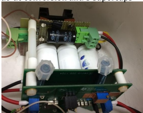
dc-dc conversion and 3 supercaps
