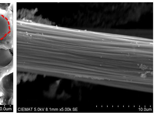
AFTER OPERATION: The morphology of fibers changes. The section is more irregular and smaller due
