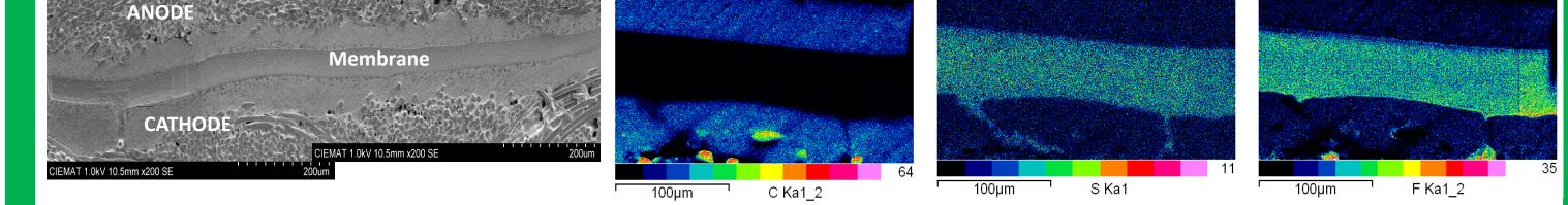
Symmetric MEA with two GDE2. After operation membrane shows different distribution of F and S. Loss of F is observed in the membrane and oxygen enrichment.
