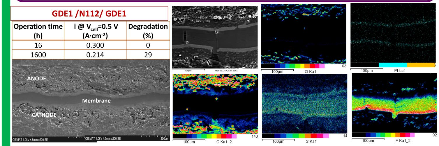
Symmetric MEA with two GDE1. Operation causes F and S concentration at the cathodic side of the membrane. Pt layer presents some thinning at the anode.
