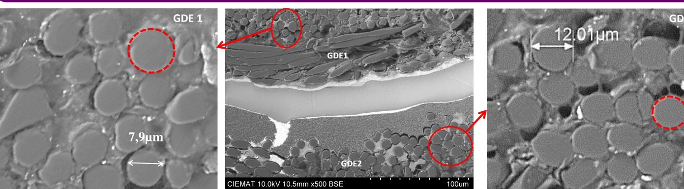
BEFORE OPERATION: The fiber section is circular, with diameters between 8 and 12 microns.
