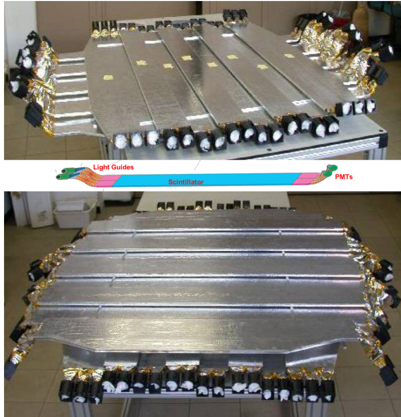
Figure 2.9: Upper and lower TOF together with a scheme of one of the paddles.
